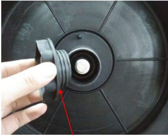
(1) Remove the spool retaining nut.
